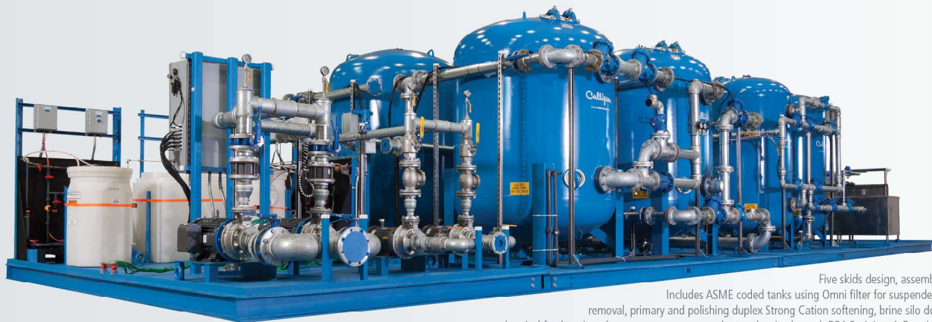
Culligan built this RO to meet a client's rigid refinery specifications, including galvanized skid, B31.3 piping, Class 1 Div. 2 Explosion Proof controls, high temperature operation at 130°F, duplex cartridge filters and duplex feed pumps with Allen Bradley PLC and HMI.
