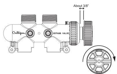
Figure 1. Bypass Position
