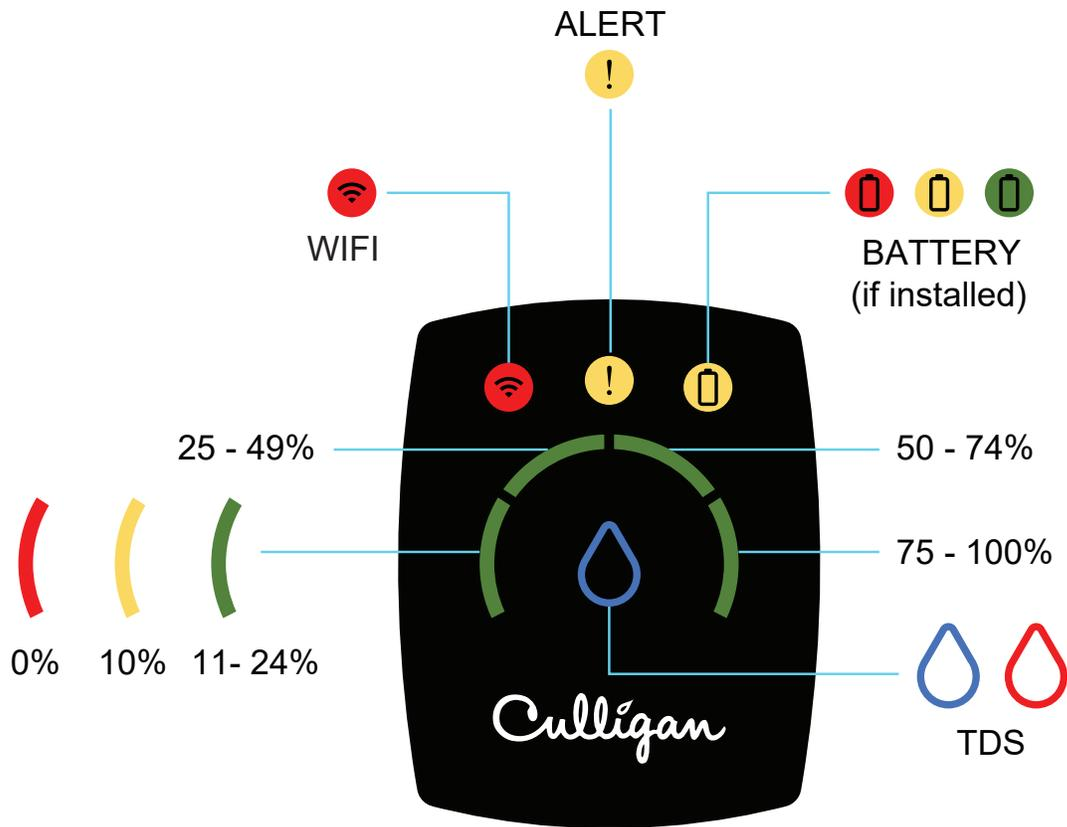
**NOTE!** Wi-Fi icon will only illuminate red if the device was previously connected, but now can no longer connect (router unplugged, changed Wi-Fi password, router has been moved too far to reach the device, etc.)
